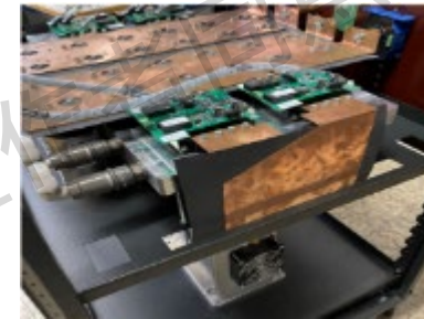
500kW DAB test equipment based on FMF1200DX1-24A
