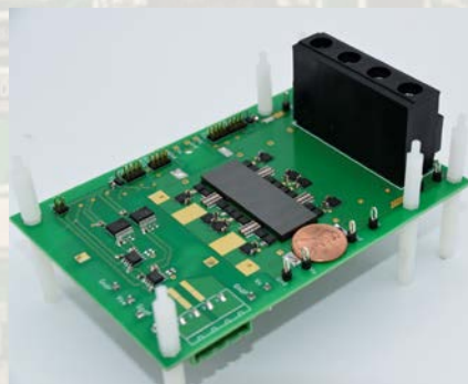
1 kW, 1 MHz, 380-12 V Server Power Supply, Circa 2021 (Mike Ranjram, MIT)
