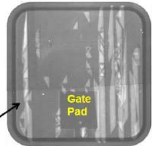
Fig. 15. Photoluminescence mapping images of stacking faults after stress of 1640 \text{ A}/\text{cm}^2 for 90 seconds
